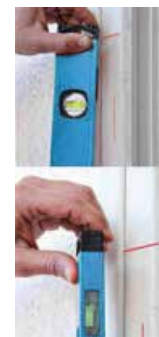
Turn the level 180° side to side
